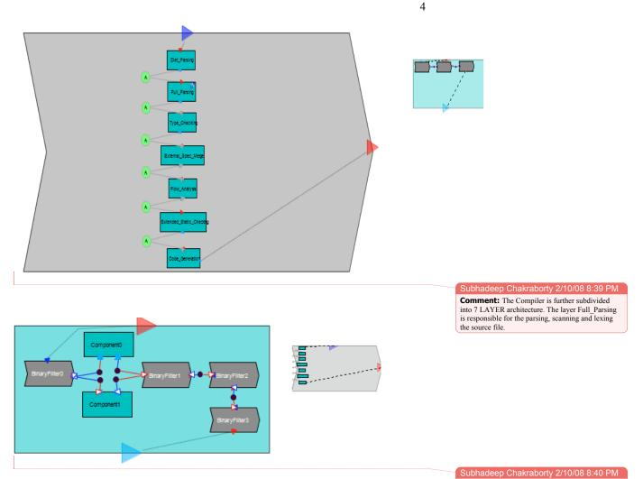
**Comment:** The innermost layer is composed of 4 Binary filters and 2 components. It is in fact a HETEROGENOUS architecture.
